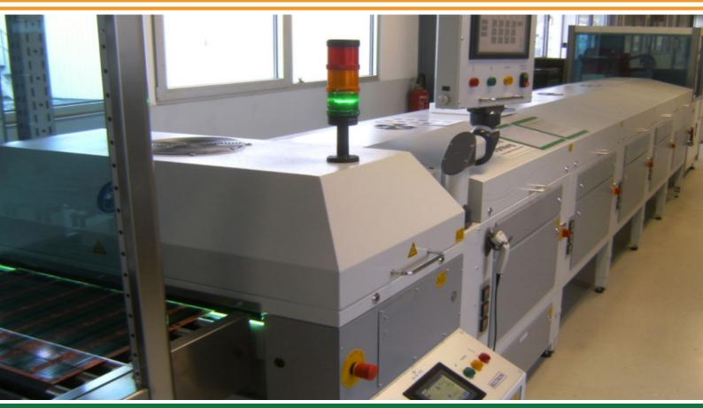
BELTROTHERM FINAL CURING PHOTO SOLDERMASK AFTER EXPOSURE AND DEVELOPEMENT WITH UV-BUMP OPERATION FIRST
