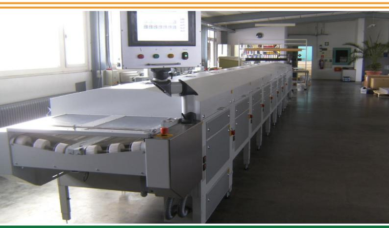
BELTROTHERM CONTINUOUS BELT DRYER FOR EVAPORATION AND DRYING AFTER WET LACQUER COATING
