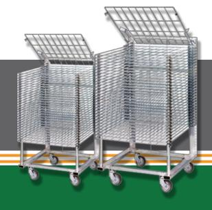
BELTRON-stacking dryer are produced in 5 different types with grid or wire netting. These stacking dryer could be built with 50, 30 or 25 galvanized drying gratings. 3 mm strong crossbars in distance of 75 mm and 4 mm strong vertical bars in distance of 200 mm produce (yield) a perfect put in and slip.
